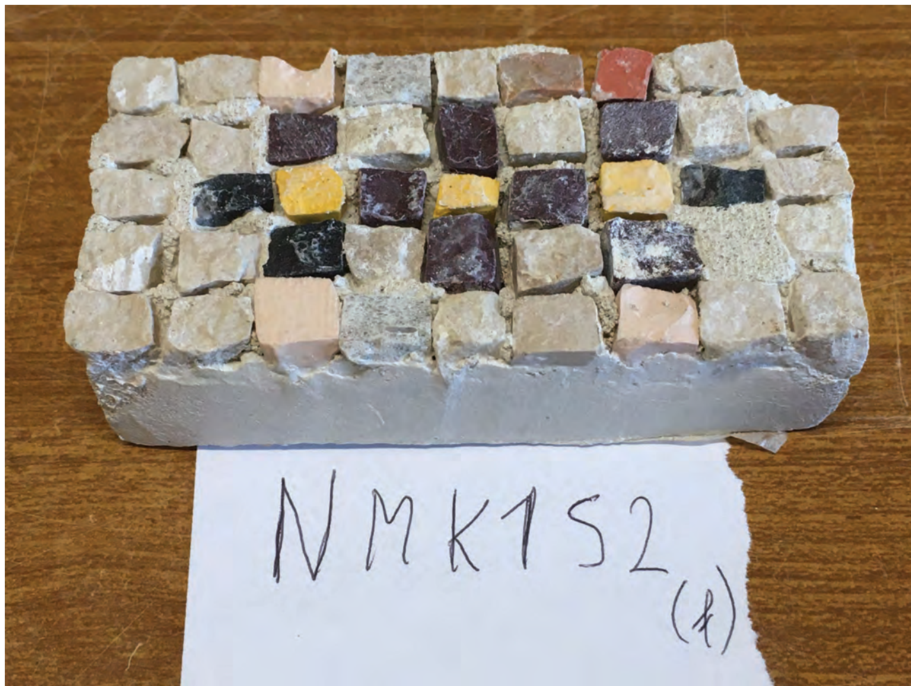
Fig. 1. Development of bedding mortars used for restoration, based on NHL and metakaolin. Laboratory tests, an example of application of bedding mortar from the back of the tesserae on a mosaic model made in reverse technique (indirect method) (photo M. Macchiarola)
